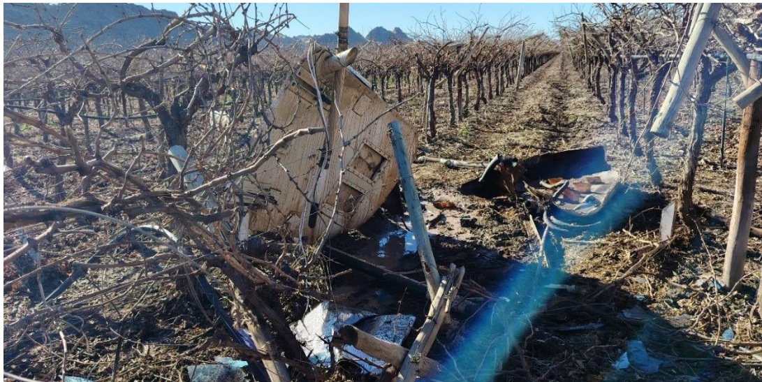
Figure 9: The lower compartment of the helicopter which housed the pesticide.
