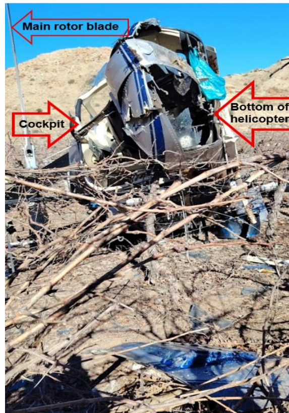
Figure 5: The damage pattern indicates that the helicopter impacted the ground in a nose-down attitude.
