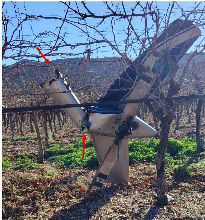
Figure 8: The tail rotor assembly found 15m from the main wreckage (the red arrows indicate the breakage points).
